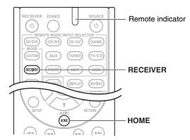
To reset the remote controller to its factory defaults, while holding down **RECEIVER**, press and hold down **HOME** until the remote indicator lights (about 3 seconds). Within 30 seconds, press **RECEIVER** again.
